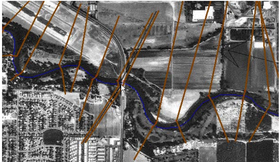
Figure 6-126. Bridges not perpendicular to the river require moving the bounding sections.
