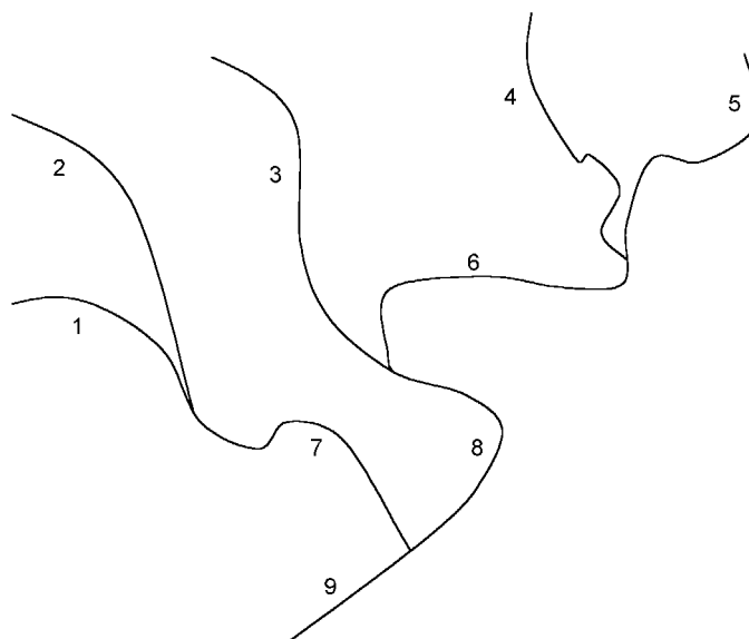
Figure 1.51 Successive computation of discharge at Kinematic Routing branches. The numbers denote the branch calculation order for a Kinematic Routing branch network.
