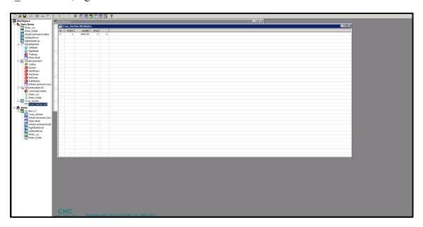
Right click on cross\_section->resample->on resample options, change method into equal distance. Select resampled cross section->tools->map object->over the whole mesh.
