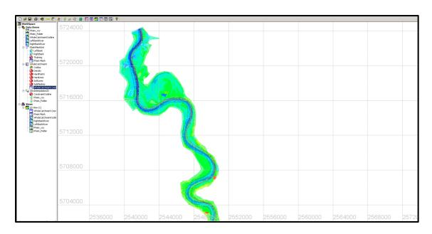
To verify that the work done is correctly, draw a new line between two points within the catchment. Select new open line, draw two points and save as cross\_section. From the cross\_section line, right click->show attribute table.
