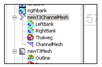
Generate new mesh for the whole domain. File->New File ->new T3 mesh generator. Click OK. Right click on the newly created mesh -> channel mesh -> metadata -> change the name to ChannelMesh
